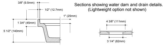
Cast Weight Specs: Gross Weight = 230 lb; Net Weight (w/Insert) = 159 lb; Net Weight (w/Turtle) = 127 lb
